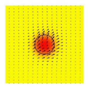
The animation this frame was taken from (q.v.) shows the development of the soliton over the course of about 2.7 nanoseconds. Current begins passing through the channel in the center, causing the magnetization to oscillate. These oscillations initially move throughout the layer, but after 1.8 ns the magnetization under the hole inverts to form the soliton (center changes to red) and the oscillations are then localized. Credit: NIST
