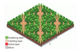
This schematic diagram of a thin film organic solar cell shows the top layer, a patterned, roughened scattering layer, in green. The organic thin film layer, shown in red, is where light is trapped and electrical current is generated. The film is sandwiched between two layers that help keep light contained within the thin film.
