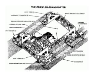
Pictured is a schematic of the crawler's design. Image credit: NASA
