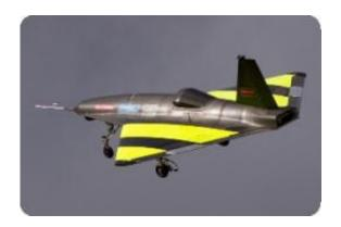
The flapless system, developed around a concept called fluidic flight control, was the result of collaborative work between Cranfield and Manchester universities together with BAE Systems' Advanced Technology Centre and was tested in wind tunnels and on models before the full-scale trials on DEMON took place.
