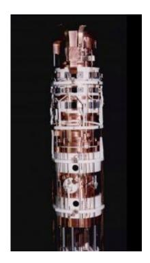
The NIST force sensor is a crystal of ions (charged atoms) trapped inside the upper region of the copper cylinder. A laser beam directed upward through the trap cools the ions. A force is applied in the form of an oscillating electric field, and a detector (not shown) measures the light reflected off the ions. Credit: Bollinger/NIST
