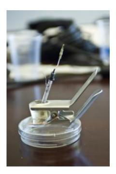
This proof-of-concept version of the photoelectrochemical cell, which was used for laboratory tests, contains a photoactive solution made up of a mix of selfassembling molecules (in a glass cylinder held in place by metal clamp) with two electrodes protruding from the top, one made of platinum (the bare wire) and the other of silver (in a glass tube). Photo: Patrick Gillooly
