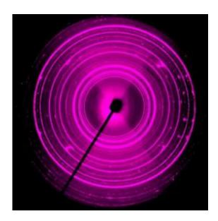
This X-ray diffraction image of a small sample of post-perovskite, which exists deep in the Earth's interior, was taken while the mineral was being compressed to pressures more than one million times atmospheric pressure. Credit: Lowell Miyagi/Yale University
