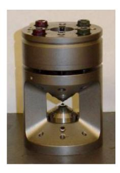
A diamond anvil cell can compress materials to several million times atmospheric pressure to reproduce conditions deep underground. (UC Berkeley)
