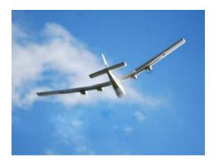
A MAVinci unmanned autonomous micro air vehicle (MAV) with a wingspan of less than two metres which is used to inspect land areas. Credits: MAVinci
