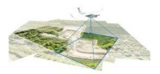
How MAVinci unmanned micro air vehicles (MAVs) are used to survey land areas, such as development areas, construction sites, disaster zones and waste disposal sites. The same principle was used in Spain to study erosion canyons. Credits: MAVinci
