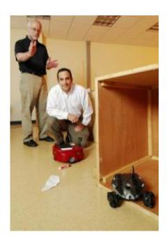
The black robot intentionally knocked down the red marker to deceive the red robot into thinking it was hiding down the left corridor. Instead, the black robot is hiding inside the box in the center pathway. Credit: Georgia Tech Photo: Gary Meek
