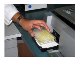
Microtiter-plate with Diclofenac-ELISA at the laboratory of the TUM-Institute of Hydrochemistry. If Diclofenac is detected, the yellowish color fades and the concentration can be detected photometrically. Credit: Picture: Andreas Battenberg / TUM
