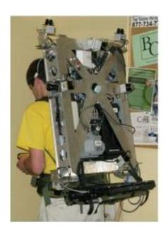
A portable, laser backpack for 3-D mapping has been developed at the University of California, Berkeley where it is being hailed as a breakthrough technology capable of producing fast, automatic and realistic 3-D mapping of even difficult interior environments. Credit: Credit: John Kua, University of California, Berkeley
