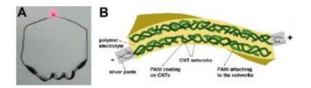
(A) Using three of the new highly flexible supercapacitors arranged in series, the researchers demonstrated lighting a red LED. (B) An illustration of the flexible, all-solid-state paper-like polymer supercapacitors. Image credit: Chuizhou Meng, et al. © 2010 American Chemical Society.
