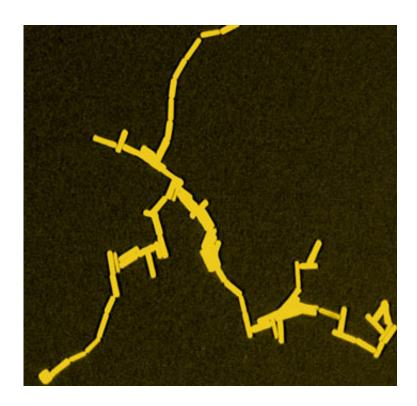
Transmission-electron-microscope image of 70-nm-long gold nanorods assembled end to end via solvent-mediated interactions.
