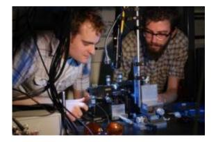
Research physicists Jonathan Matthews (left) and Kostas Poulios aligning the quantum optical chip. The photons are injected into the chip using optical fiber and requires precision alignment. Credit: Photograph by Dirk Dahmer
