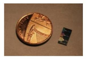
This is the photonic chip next to a UK penny. The chip contains micrometer and sub-micrometer features and guide light using a network of waveguides. The output of this network can be seen on the surface of the chip. Credit: Photograph by Jasmin Meinecke
