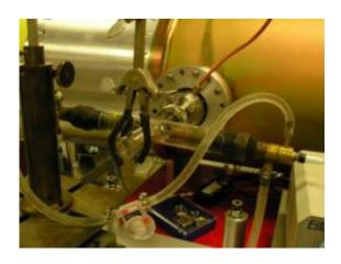
NIST's unique "sliding spark source" (inside the glass tubing) feeds ultraviolet light into NASA's Solar Ultraviolet Magnetograph Investigation instrument, designed to measure magnetic fields on the sun. Credit: Reader/NIST
