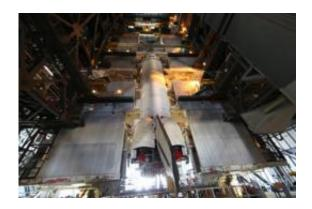
Space shuttle Discovery inside the cavernous Vehicle Assembly Building. Work platforms are lowered all around the spacecraft to give technicians access to the various systems and components as they attach the orbiter to the rest of the stack and prepare it for launch. Discovery is targeted for launch Nov. 1 on the STS-133 mission. Photo credit: NASA/Dimitri Gerondidakis
