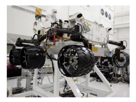
Engineers working in a clean room at NASA's Jet Propulsion Laboratory, installed six new wheels on the Curiosity rover, and rotated all six wheels at once on July 9, 2010. Iredit: NASA/JPL-Caltech
