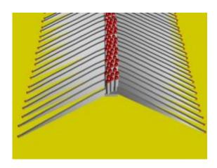
Graphic illustrates a single row of nanowires (cylinders with red tops) with finshaped nanowalls extending outward. The transmission electron microscope image shows four rows of nanowires and their corresponding nanowalls, nicknamed "nano LEDs" because they emit light when electrically charged. The distance across the micrograph is approximately the diameter of a human hair. Credit: NIST
