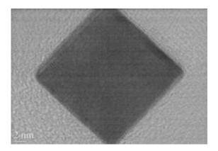
These electron microscope images show perfect-edged nanocubes produced in a one-step process created at NIST that allows careful control of the cubes' size, shape and composition. Credit: NIST
