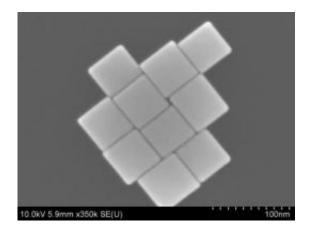
These electron microscope images show perfect-edged nanocubes produced in a one-step process created at NIST that allows careful control of the cubes' size, shape and composition. Credit: NIST
