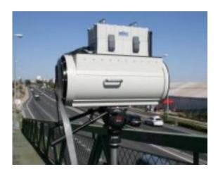
This is an image of the one of the parts which detect pollution on the roads. Credit: UC3M
