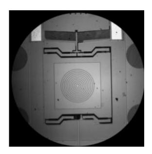
This is the NIST MEMS-based rheometer. The moving plate is controlled by resistance heating elements in the chevron-like structure at the top; expansion and contraction of the vanes causes the plate to move up and down. Central square where the sample would rest is approximately 500 micrometers across. Credit: Christopher/NIST
