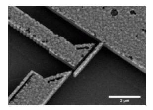
SEM image of a released SiC NEMS switch with 3  $\mu$ m length. Image credit: Science, DOI:10.1126/science.1192511
