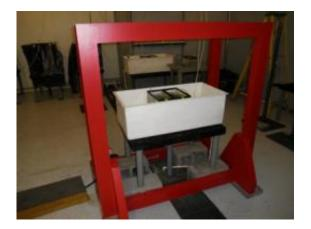
PNNL's Marine Sciences Laboratory in Sequim, Wash., has this experimental setup to expose aquatic animals to an electromagnetic field created by the two large red Helmholtz coils pictured here. The field is similar to those created by marine power devices installed in the ocean. Credit: Pacific Northwest National Laboratory
