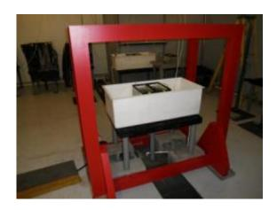
PNNL's Marine Sciences Laboratory in Sequim, Wash., has this experimental setup to expose aquatic animals to an electromagnetic field created by the two large red Helmholtz coils pictured here. The field is similar to those created by marine power devices installed in the ocean. Credit: Pacific Northwest National Laboratory
