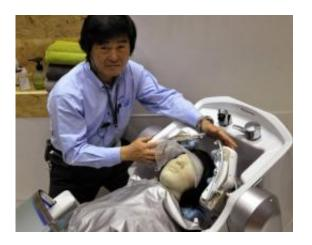
Panasonic robot development engineer Tohru Nakamura displays the new robot hairwasher, which scans a client's head using 3D technology, then shampoos their hair and massages the scalp with its rubbery "fingers".
