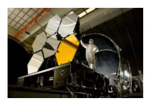
Ball Aerospace optical technician Scott Murray inspects six primary mirror segments, critical elements of NASA's James Webb Space Telescope, prior to cryogenic testing in the X-ray & Cryogenic Facility at NASA's Marshall Space Flight Center in Huntsville, Ala. The James Webb Space Telescope will be launched in 2014 to study the formation of the first stars and galaxies and shed new light on the evolution of the universe. (NASA/MSFC/David Higginbotham)
