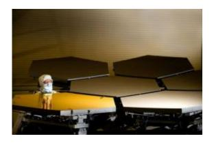
Ball Aerospace lead optical test engineer Dave Chaney inspects the first gold primary mirror segment, a critical element of NASA's James Webb Space Telescope, prior to cryogenic testing in the X-ray & Cryogenic Facility at NASA's Marshall Space Flight Center in Huntsville, Ala. The James Webb Space Telescope will be launched in 2014 to study the formation of the first stars and galaxies and shed new light on the evolution of the universe. (NASA/MSFC/David Higginbotham)
