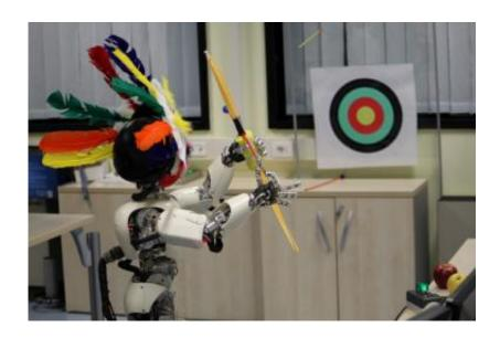
Humanoid robot iCub learns the skill of archery. The learning algorithm, called ARCHER (Augmented Reward Chained Regression) algorithm, was developed and optimized specifically for problems like the archery training. Photo: Dr. Petar Kormushev
