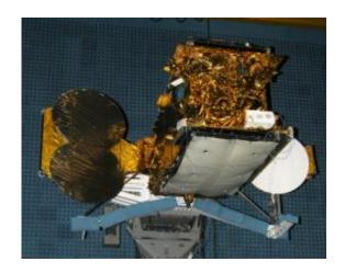
Hylas-1 during qualification testing at the Compact Antenna Test Facility (CATF) at ISRO's Bangalore satellite centre. Credits: ISRO
