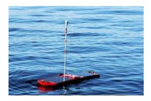
This undated handout photo provided by BP, shows a Wave Glider, a new type of robotic boat measuring water quality and doing scientific research for BP. It is satellite controlled, gets its propulsion power from wave action, and uses solar power to run its scientific electronics. (AP Photo/BP)
