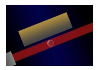
A beam of laser light (red) should be able to cause a glass bead of approximately 300 nanometers in diameter to levitate, and the floating bead would be exquisitely sensitive to the effects of gravity. Moving a large heavy object (gold) to within a few nanometers of the bead could allow the team to test the effects of gravity at very short distances. Credit: K. Talbott/NIST
