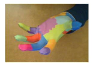
The colors are printed on a Lycra fabric glove that contains no sensors. The unique color pattern is designed to help robust tracking of the hand.
