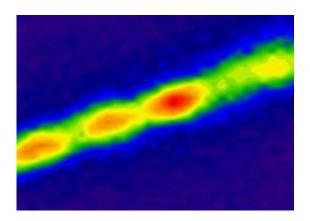
This filament containing about 30 million carbon nanotubes absorbs energy from the sun as photons and then re-emits photons of lower energy, creating the fluorescence seen here. The red regions indicate highest energy intensity, and green and blue are lower intensity. Image: Geraldine Paulus
