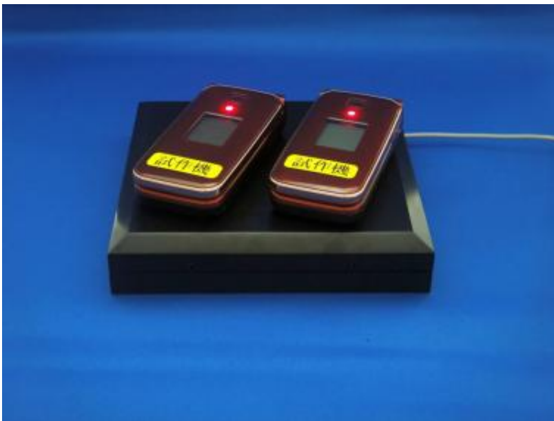
Figure 2. Prototype mobile phones with built-in wireless power receivers
