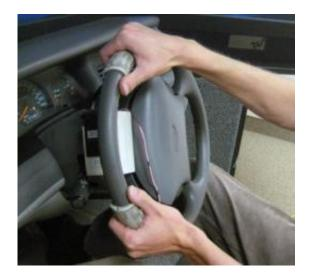
Two devices, mounted on the steering wheel of a driving simulator, convey navigation information (turn left or turn right) to the driver. The driver's index fingertips rest on two IBM ThinkPad TrackPoint buttons (not visible) that move left or right by about 1 millimeter (a twenty-fifth of an inch) to tell the driver which way to turn. Credit: Nate Medeiros-Ward, University of Utah.
