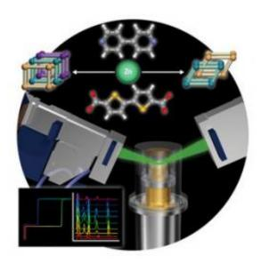
Schematic representations of the synthesis of the two-fold and three-fold interpenetrated porous coordination polymers, structural analysis by x-ray powder diffraction and adsorption and desorption profiles. Copyright: 2010 Ryotaro Matsuda
