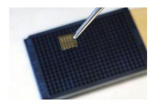
The new electronic microplate is shown in front of the technology it aims to replace, the conventional microplate. Credit: Gary Meek
