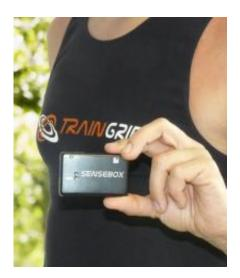
TrainGrid consists of an e-shirt with sensors to determine in real time the athlete's electrocardiogram, heart rate, skin temperature, body position and location via satnav. All the data are transmitted via Bluetooth to a mobile phone or computer to share with a coach, doctor, friends or on a social network. Credits: emxys
