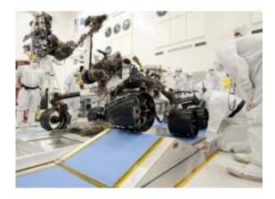
The suspension system on NASA Mars rover Curiosity easily accommodates rolling over a ramp in this Sept. 10, 2010, test drive inside the Spacecraft Assembly Facility at NASA's Jet Propulsion Laboratory, Pasadena, Calif. Image Credit: NASA/JPL-Caltech
