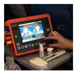
The briefcase-sized Tempus IC telemedicine system puts non-medical cabin crew in contact with ground-based experts during in-flight medical emergencies. Key information about the passenger's health can be quickly transmitted via satellite to a dedicated response centre. The same vital signs which are measured
