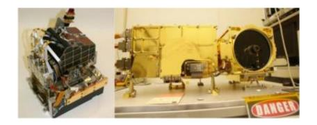
The two main parts of the ChemCam laser instrument for NASA's Mars Science Laboratory mission are shown in this combined image. Image Credit: NASA/JPL-Caltech/LANL
