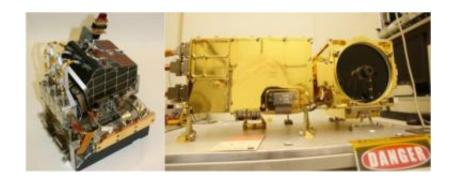
The two main parts of the ChemCam laser instrument for NASA's Mars Science Laboratory mission are shown in this combined image. Image Credit: NASA/JPL-Caltech/LANL
