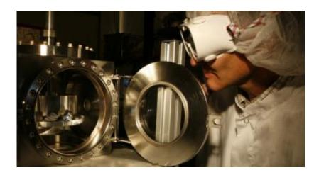
The ChemCam instrument for NASA's Mars Science Laboratory mission uses a pulsed laser beam to vaporize a pinhead-size target, producing a flash of light from the ionized material -- plasma -- that can be analyzed to identify chemical elements in the target. Image Credit: NASA/JPL-Caltech/LANL
