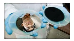
A silver wafer reflects the face of NREL research scientist Hao-Chih Yuan, before the wafer is washed with a mix of acids. The acids etch holes, absorbing light and turning the wafer black. Credit: Dennis Schroeder
