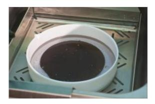
The process takes just three minutes at room temperature. Inside a laboratory at NREL's Solar Energy Research Facility, an acid mixture bubbles atop a silicon wafer as it etches holes and works toward turning the wafer black. Credit: Dennis Schroeder
