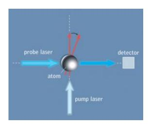
In a vapor-cell magnetometer, the spin of a population of atoms is first polarized, as indicated by the vertical red arrow, by a pump laser that is itself circularly polarized. When a magnetic field is applied, the spin vector is rotated, as indicated by the tilted red arrow. (The magnetic field is perpendicular to the plane of this diagram.) The probe laser's own plane polarization is rotated by the atom's spin, and the degree of rotation is measured at the detector.
