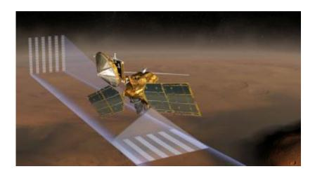
This artist's concept shows NASA's Mars Reconnaissance Orbiter, whose Mars Climate Sounder instrument has been profiling the Martian atmosphere for four years. The instrument has just begun a campaign to examine atmospheric conditions for the Martian season and hour when the next Mars rover will land in 2012.
