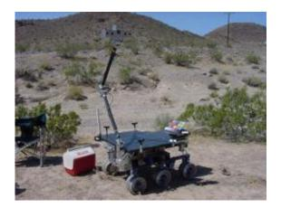
Testing the MER-FIDO rover in the field, April 30 - May 9, 2001. The design for the Mars Exploration Rovers was subjected to many tests at field sites on Earth. Image credit: Department of Earth and Planetary Sciences, Washington University in St. Louis
