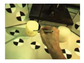
Real or virtual? The virtual object, in this case the white cylinder, is projected into the actual environment and can be felt using a sensor rod. (Picture: Matthias Harders / ETH Zurich)
