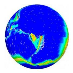
Plate boundaries, which can be seen as narrow red lines are resolved using an adaptively refined mesh with 1km local resolution. Shown are the Pacific and the Australian tectonic plates and the New Hebrides and Tonga microplates. Credit: Georg Stadler, Institute for Computational Engineering & Sciences, UT Austin
