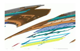
Exploded view of the air shutter system in the 2011 Chevrolet Cruze which uses sensors to feel and sense wind and temperature conditions. The sensors work with electric motors that open and close shutters automatically, contributing nearly half a mile per gallon in combined city and highway driving.
