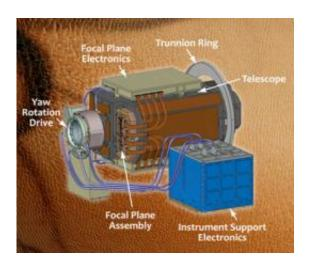
The UA's High Resolution Stereo Color Imager, or HiSCI, features an innovative rotation drive for three-dimensional imaging. As the instrument orbits the Red Planet, it snaps pictures once a feature of interest on the surface below comes into view. HiSCI then swings around and takes more pictures of the feature as it passes overhead.
