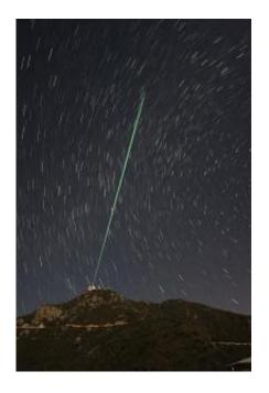
A bundle of laser beams creates five artificial stars in the night sky above Mount Hopkins in Southern Arizona. Laser light reflected by air molecules is analyzed by a computer that drives the actuators on the adaptive mirror. Credit: (Image courtesy of Thomas Stalcup)
