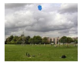
The kite retrieves wind speed measurements by sensing the tension in the tether that is connected to the ground.
