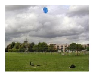
The kite retrieves wind speed measurements by sensing the tension in the tether that is connected to the ground.
