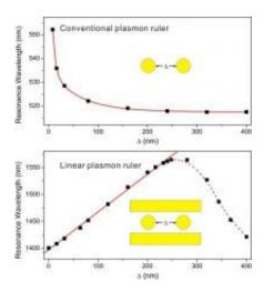
In contrast to a conventional nanoparticle dimer plasmon ruler, this new one shows an approximately linear relationship between the resonance wavelength shifts and nanosphere dimer interparticle separation for a linear plasmon ruler.
